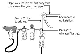
Place a drain trap at low points to remove water. Also utilize on main line at low points.
